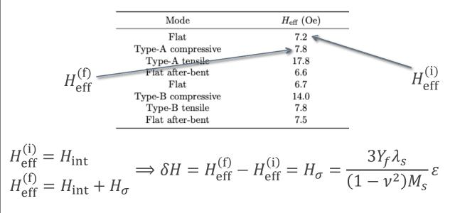
Flexible EPHE sensors can measure both magnetic fields and strains simultaneously **under the application of an external field.**
