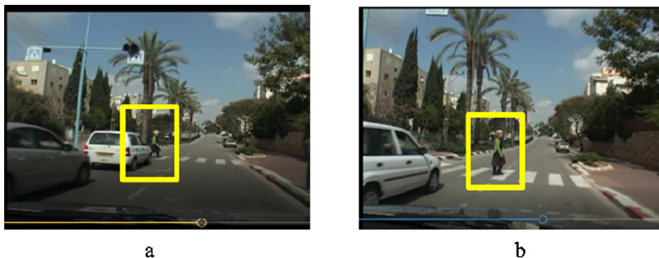
Fig. 5. Representative frames of the hazard (pedestrian crossing the road started obscured by a stopping car and eventually becoming full visible) in Movie TR-08, (a) 4700 ms and (b) 6000 ms after the initial appearance of the hazard's precursor, corresponding to the estimated NRT of trained (a) and untrained (b) driver groups.
